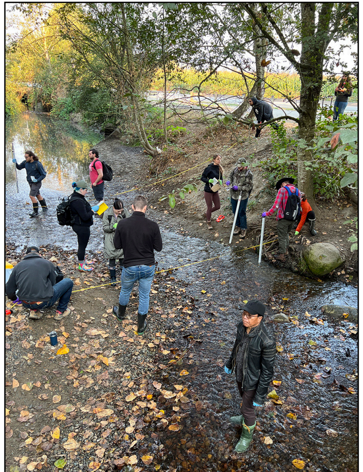
Measuring the dimensions of the creek channel with tapes and survey rods
